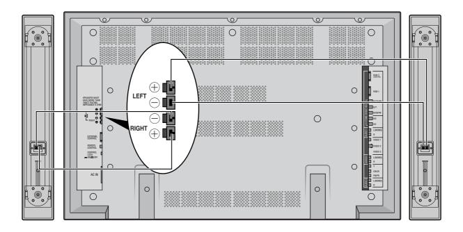
External speakers may be connected to the plasma monitor to reproduce sound from VIDEO, DVD or RGB signal sources.
